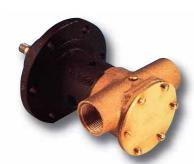
Flexible vanes create increased volume when leaving the eccentric cam creating a vacuum thus drawing in liquid, instantly priming the pump.
