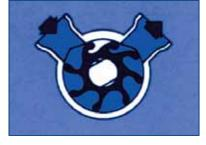
As the flexible vanes rotate, the liquid is carried through the pump from the inlet to outlet port, each successive vane drawing in liquid.
