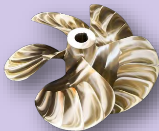
High speed passenger ship propeller Diameter:1.6m, weight:500kgs
