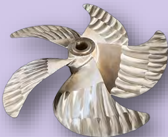
Large container ship propeller Diameter:5.6m, weight:9.8tons
