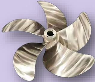
Large container ship propeller Diameter:4.8m, weight:9tons
