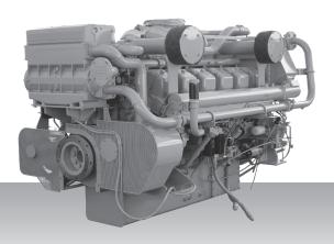
12-cylinder, 4-cycle, water cooled diesel engine, with direct-injection, turbocharger, air-cooler, built-up heat exchanger and sea water pump.
