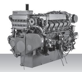
12-cylinder, 4-cycle, water cooled diesel engine, with direct-injection, turbocharger, air-cooler, built-up heat exchanger and sea water pump.
