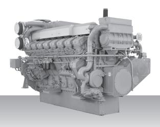
16-cylinder, 4-cycle, water cooled diesel engine, with direct-injection, turbocharger, air-cooler, built-up heat exchanger and sea water pump.
