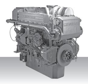
6-cylinder, 4-cycle, water cooled diesel engine, with direct-injection, turbocharger, air-cooler, build-up heat exchanger and sea water pump.
