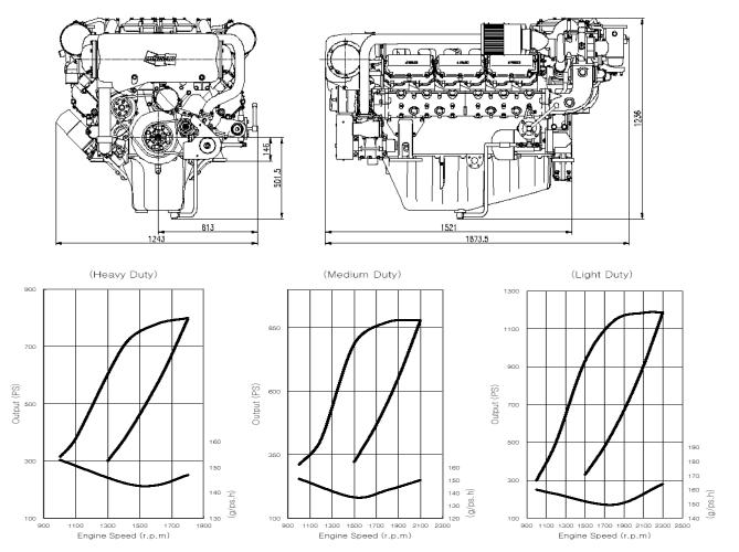
Heavy Duty : Operation hours are unlimited per year, at average load is up to 90 %, at full load is up to 80 % Typical gearbox ratio: 2.5 ~ 6
